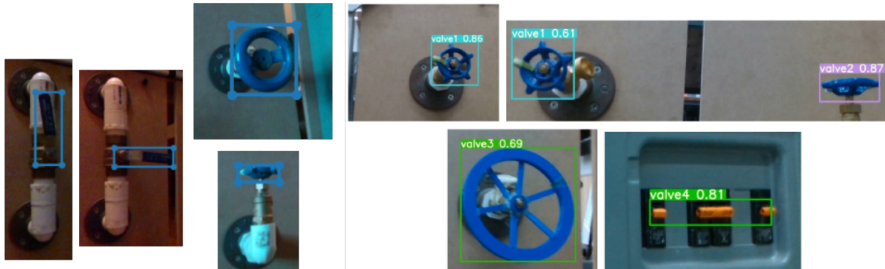
Figure 17: Training and inferred samples. The left four images show training samples along with state-classes for standing valve. On the right is the detection from the model with prediction score
