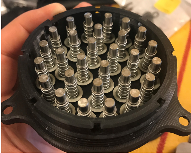
Figure 13: An image of the inner enclosure that housed all of the springs/pins. A cover went over this enclosure to load the springs.
